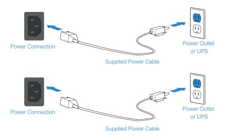
Plug in your device to a power outlet using the provided power cables.
