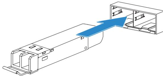
5. Press the transceiver firmly into the cage socket with your thumb.
