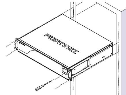
4. Finger tighten four rack-mount screws to attach the unit to the rack.
