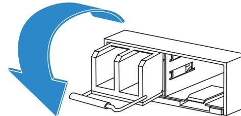
5. Replace the cap on the SFP cage socket and place the removed SFP transceiver into an antistatic bag.
