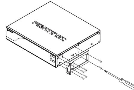
2. Position the FortiGate unit in the rack. Ensure there is enough room around the unit to allow for sufficient air flow.
