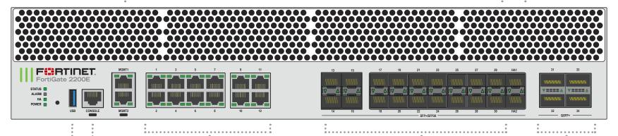
USB (USB A) ← USB 3.0 server port Ethernet Ports 1 to 12 (RJ-45)
