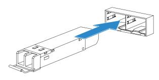
5. Press the transceiver firmly into the cage socket with your thumb.
