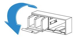
5. Replace the cap on the SFP cage socket and place the removed SFP transceiver into an antistatic bag.
