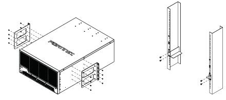
5. Ensure there is enough room around the unit to allow for sufficient air flow, then secure the device to the rack with rack-mount screws.
